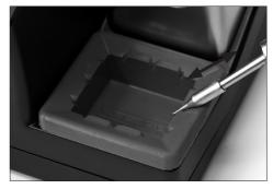
Use the slots to wipe any posible particle sticked on the tip
