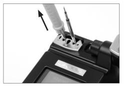
Pull slightly to remove the cartridge
