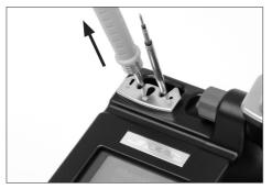
Pull slightly to remove the cartridge
