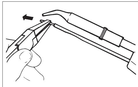
The solder flux may cause clogging at the end of the guide tube: clean when necessary.
