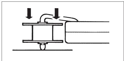
Before fitting a new reel, pull out the solder remaining inside the tube.
